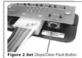
Figure 2 Set Stops/Clear Fault Button
