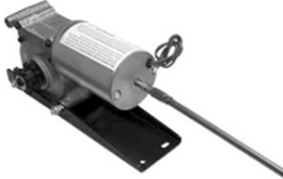
3. Attach 1/4" socket & ratchet, or drill to the other end, and turn in the proper direction to move the room.
