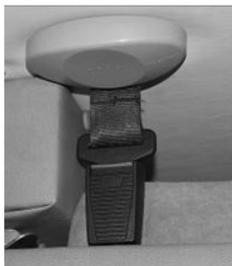
**Fig.1 Belt Interlock Latched**
