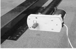
Fig. 3-Hex Head Crank Extension
