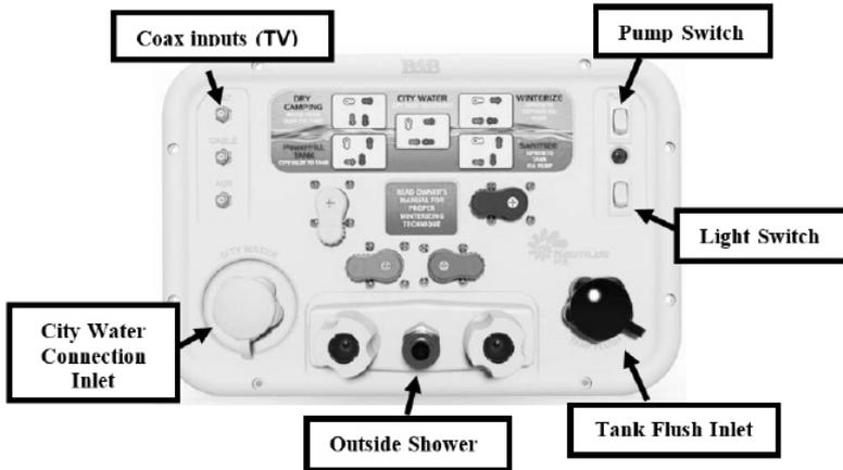
The **Uni-Doc Utility Center** is located in an exterior compartment and allows you to perform the following functions:
